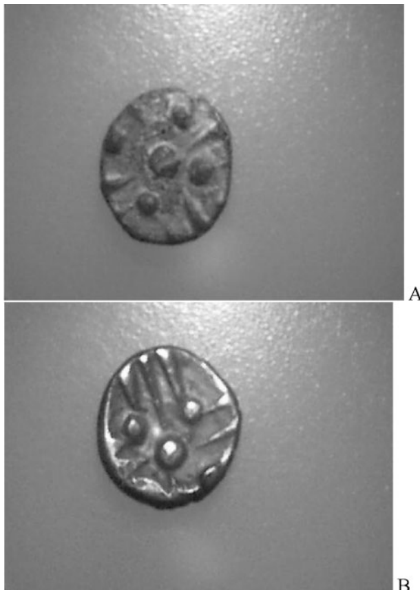
4 a Ancient fake of a Celtic silver drachma , made of 65% tin, 24% copper, 1.5% silver and 3.5% lead. b Authentic Celtic drachma . Celtic drachmae are made of silver with only ca. 2–6% copper. (Photo: A. Giumlia-Mair)
